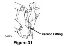
3. Install a grease gun onto the fitting and gently apply 2 or 3 pumps of #2 multipurpose lithium base grease (Fig. 31).
